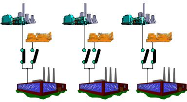
The open transition transfer removes power to the load when it switches from one source to another.
