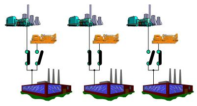
The soft-load transfer is similar to a "closed transition" except that the transfer is made without any detectable change to the downstream voltage.
